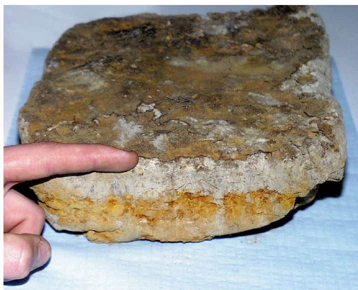
Figure 4.37. Iron-rich crust composed of schwertmannite, ferrihydrite and goethite derived from the oxidation and dissolution of the sulfide framboids in an acid sulfate soil from Guthries. The layers are described in Figure 5.18.
